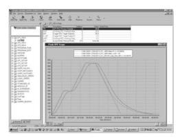
Eurotherm's advanced control algorithm gives precise straight-line control. Automatic tuning simplifies the commissioning procedure by performing a one shot tune to calculate the optimum PID values. To further optimise control especially in programmer applications, gain scheduling can be used to transfer control between up to six sets of PID values.
