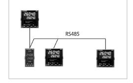
Master Modbus communications significantly increases the applications open to the 2604 controller. In its simplest form it can be used to retransmit a setpoint to a number of slave controllers in a multizone furnace.
