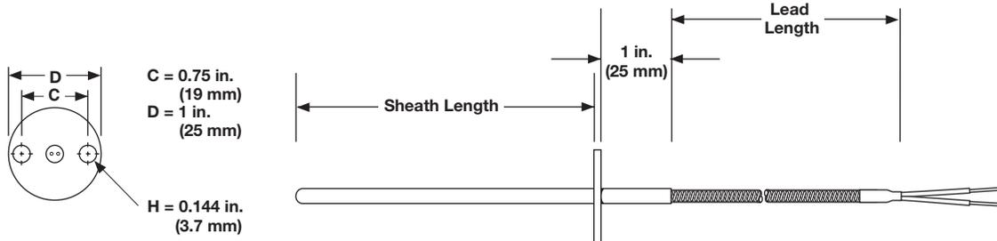
The flanged thermocouple allows rapid assembly and low profile when going through bulkheads.
