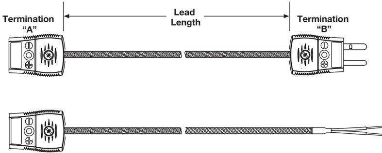
Flexible extensions allow thermocouples to be disconnected from a system without disturbing the remaining wiring.
