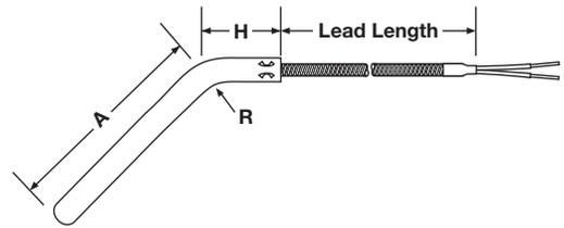
The bent rigid tube offers protection and accurate lead placement around machinery.
