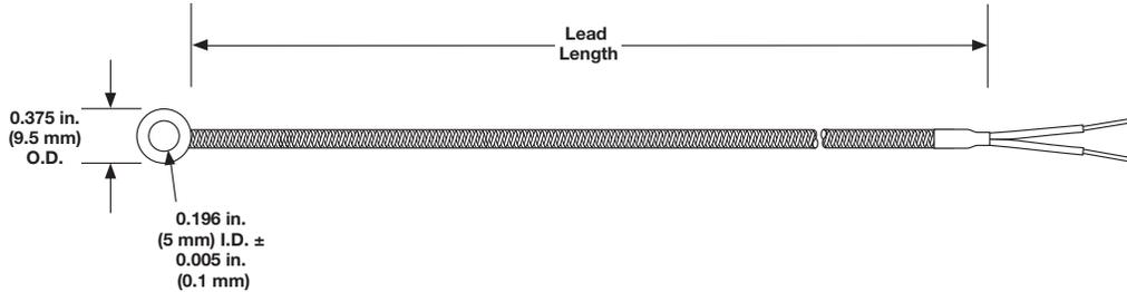
The extremely low profile of the stainless steel grommet provides fast response time.
