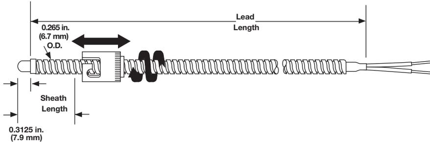
Adjustable armor thermocouples bend to any angle to fit a wide range of hole depths, eliminating the need to stock numerous styles. A stainless steel hose offers additional lead protection in demanding applications.
