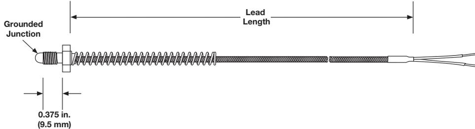
The nozzle thermocouple has a short installation depth and a low profile to allow control of thin platen sections.
