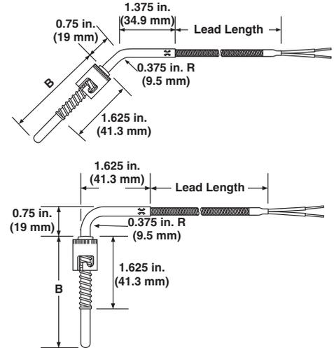
Bayonet fittings allow rapid attachment. Spring pressure on the junction tip assures fast response time.
