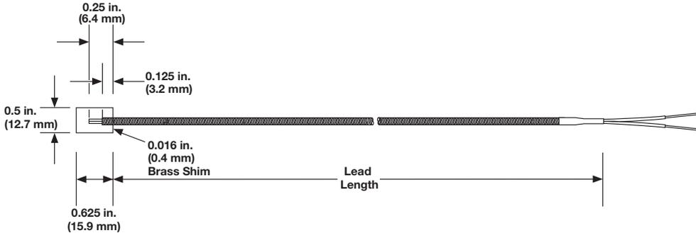
The shim stock thermocouple has a low profile and can be placed between components for surface temperature measurement.
