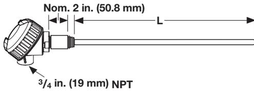
**Type 3** - 1/2 x 3 inch steel pipe nipple typical
