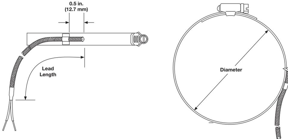
The stainless steel clamp allows temperature measurement without drilling or tapping, which is ideal for measuring pipe temperatures.
