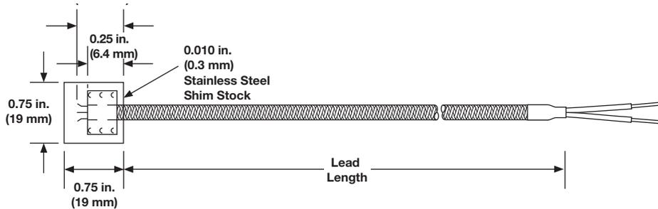
The shim stock thermocouple has a low profile and can be placed between components for surface temperature measurement.
