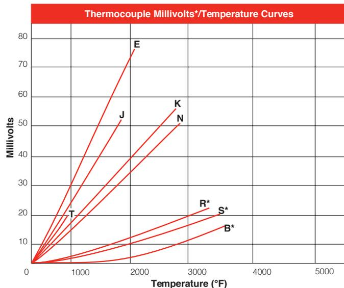
\*Millivolt values shown for R and S calibrations pertain to thermocouple calibrations only. RX and SX constructions described in this catalog section are intended for use as **extension wire only** and will not exhibit the millivolt outputs shown.
