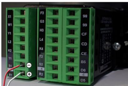
Figure 2: Thermocouple Input Wiring Example
