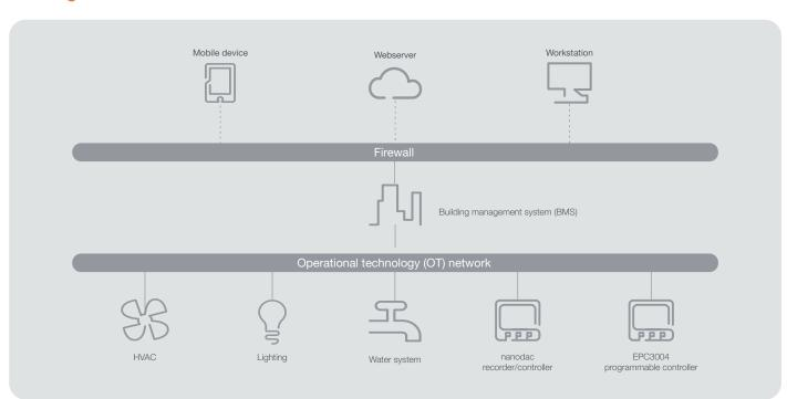
BACnet™ is widely used in heating, ventilation and air conditioning (HVAC), institutional hot water, and district energy networks. Eurotherm offers native BACnet/IP communication option on some controller and hybrid data recorder/controller ranges, via the onboard RJ45 connection.
