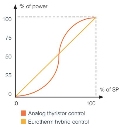
Eurotherm digital thyristor power control helps to provide linear control across the entire output % range, whereas the analog thyristor is non linear over the setpoint (SP) range.
