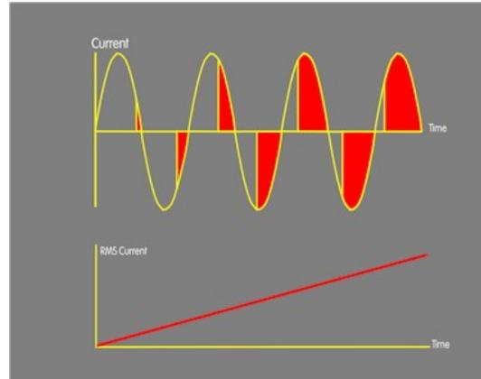
**Fig 4. Phase angle control with soft start**
