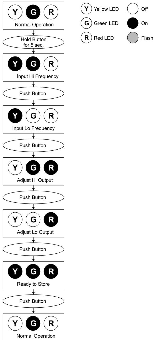
Figure 1: Q476 Calibration Flow Chart
